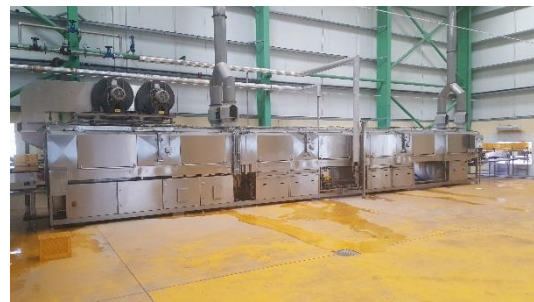
6000 PER HOUR PRE WASH/ HOT WASH HOT RINSE AIR KNIFE BLOWERS
